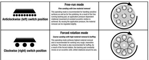
**Note:** To determine the sanding mode the sander is currently set to, disconnect the tool from the power supply, and attempt to turn the Hook and loop backing pad (I) by hand. If the pad is hard to turn and moves on an eccentric orbit, Forced rotation mode is selected. If the base turns easily around its axis, the sander is set to Freerun mode.
